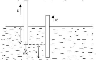
At equilibrium position, the body sinks to a height, h, below the liquid surface Up thrust = weight of the body
