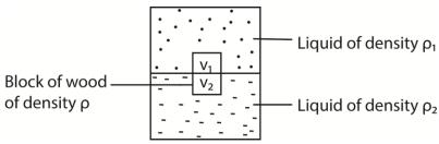
A block of wood of density  $\rho$  floats at the interface between immiscible liquids of densities  $\rho_1$  and  $\rho_2$  as shown in the figure above.
