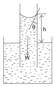
A capillary tube of radius, r, is vertically placed in a liquid. The liquid rises until the vertical component of the upward forces due to surface tension is equal to the weight of the liquid column.
