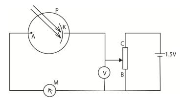
P is a vacuum photocell with anode, A, and cathode, K, made from the same metal of work function 2.0eV. The cathode is illuminated by monochromatic light of constant intensity and wavelength  $4.4 \times 10^{-7} \text{m}$
