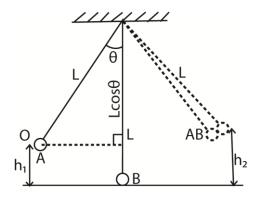
Let  $h_1$  be the height of A above the ground when the string is inclined at an angle  $\theta$  to the vertical
