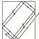
When radiation enters a black container through a hole, it undergoes multiple reflections. At each reflection, part of the radiation is absorbed. After several reflections, all the radiation is retained inside the container. Hence it approximates to a black body.
