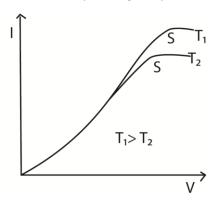
The current increases with the positive anode potential as far as the point S. Beyond this point the current does not increase, because the anode is collecting all the electrons emitted by the filament; the current is said to be saturated. More electrons are emitted at a higher temperature  $T_1$  than  $T_2$ .
