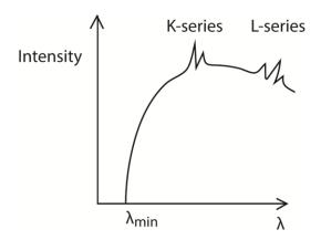
The spectrum consists of two major components, i.e. the continuous (background) spectrum and the very sharp line spectrum superimposed onto the background spectrum.
