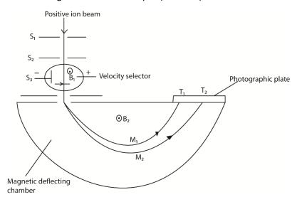
T<sub>1</sub> and T<sub>2</sub> are tracers on photographic plate, S<sub>1</sub>, S<sub>2</sub> and S<sub>3</sub> are slits
