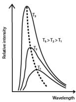
As temperature increases, the intensity increases. The intensity of shorter wavelengths increase more rapidly. The wavelength of the most intense radiation decreases as temperature increases.
