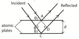
For constructive interference to occur, the path difference is equal to the whole number of wavelength
