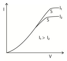
The current increases with the positive anode potential as far as the point S. Beyond this point the current does not increase, because the anode is collecting all the electrons emitted by the filament; the current is said to be saturated.
