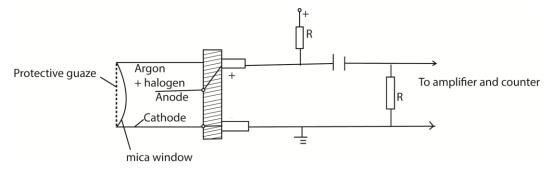
The thin mica window allows the passage and detection of the weak penetrating alpha particles. The GM tube is first evacuated then filled with Neon, Argon plus Halogen gas which is used as a quenching agent.
