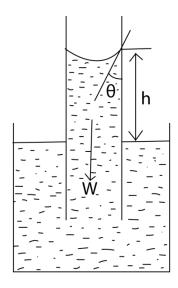
The liquid rises until the vertical component of the upward forces due to surface tension is equal to the weight of the liquid column.
