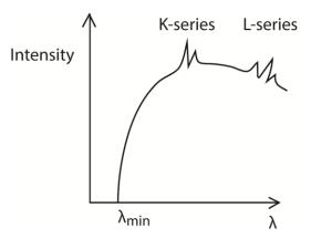
The spectrum consists of two major components, i.e. the continuous (background) spectrum and the very sharp line spectrum superimposed onto the background spectrum.
