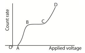
OA – the operating voltage is not enough to attract the ions to the respective electrodes and hence the counter registers no reading. This voltage (i.e. at A) is called the threshold voltage.
