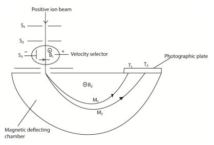
$T_1$  and  $T_2$  are tracers on photographic plate,  $S_1$ ,  $S_2$  and  $S_3$  are slits
