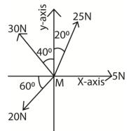
A body, M, of mass 6kg s acted on by forces of 5N, 20N, 25N and 30N as shown in the figure above. Find the acceleration of M (05marks)
