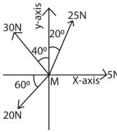
A body, M, of mass 6kg s acted on by forces of 5N, 20N, 25N and 30N as shown in the figure above. Find the acceleration of M (05marks)
