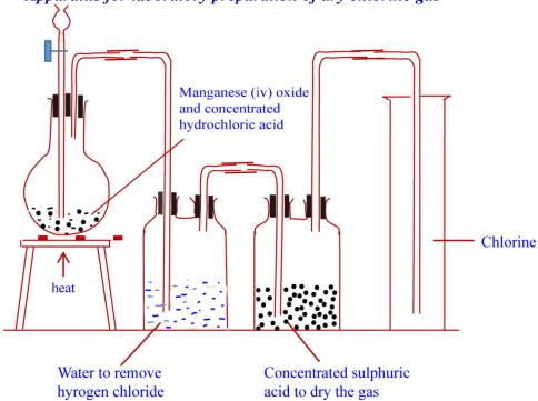
Note that chlorine is collected by downward delivery or upward displacement of air because it is denser than air
