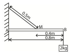
The beam is held in a horizontal position by a light inextensible string of length 0.5metres. the string joins the mid-point M of the beam to a point C vertically above A.
