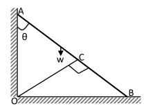
Find (i) tension in the string (ii) reaction at A and B in terms of  $\theta$  and w.
