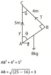
Let T be tension in the string, from the diagram  $\cos \theta = \frac{3}{5}, \cos \alpha = \frac{4}{5}$ Equation of moment about A T x 3 = 8g x 1.5cos $\alpha$ 3T = 8 x 9.8 x  $\frac{4}{5}$ ; T = 31.36N  $\therefore$  tension in the string is 31.36N (b) Magnitude of the normal reaction at A. (02marks)
