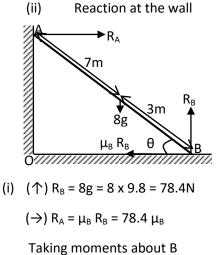
$\begin{array}{l} R_{A} \mbox{ x 10sin}\theta = 8g \mbox{ x 3cos}\theta \\ R_{A} \mbox{ x 10sin}30 = 8g \mbox{ x 3cos 30} \\ R_{A} = \mbox{ 40.738N} \\ \mbox{ Reaction at the wall = 40.738N} \\ R_{A} = \mbox{ } \mu_{B} \mbox{ } R_{B} = 78.4 \mbox{ } \mu_{B} \\ \mbox{ 78.4 } \mbox{ } \mu_{B} = 40.738 \\ \mbox{ } \mu_{B} = 0.5196 \end{array}$
