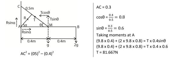
(b) Magnitude and direction of the force exerted by the hinge. (04marks) Resolving forces
