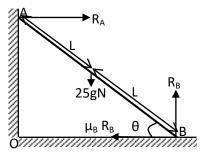
(i) ( $\uparrow$ ) R<sub>B</sub> = 25g = 25 x 9.8 = 245N ( $\rightarrow$ ) R<sub>A</sub> =  $\mu_B$  R<sub>B</sub> = 245  $\mu_B$ Taking moments about B R<sub>A</sub> x 2Lsin $\theta$  =25g x Lcos $\theta$
