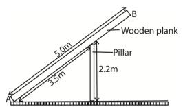
Given that the coefficient of friction at the ground is 0.6and the plank is just to slip, find the
