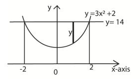
A of the curve and x-axis =  $\int_{-2}^{2} y dx = \int_{-2}^{2} (3x^2 + 2) = [x^3 + 2x]_{-2}^{2} = (8 + 4) - (-8 - 4) = 24$ Total area of the rectangle = 4 x 14 = 56 Area of the curve and the line (y = 14)
