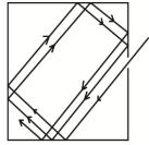
When radiation enters a black container through a hole, it undergoes multiple reflections. At each reflection, part of the radiation is absorbed. After several reflections, all the radiation is retained inside the container. Hence it approximates to a black body.
