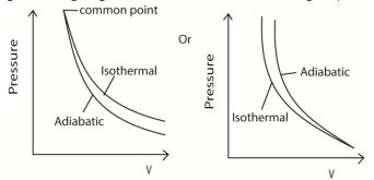
(b) An ideal gas is trapped in a cylinder by a movable piston. Initially it occupies a volume of 8 x 10<sup>-3</sup>m<sup>3</sup> and exerts a pressure of 108kPa. The gas undergoes an isothermal expansion until its volume is 27 x 10<sup>-3</sup>m<sup>3</sup>. It is then compressed adiabatically to the original volume of the gas. (i) Calculate the final pressure of the gas (06marks)
