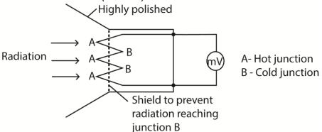
Radiation falling on junction A is absorbed and temperature rises above that of junction B. An e.m.f is generated and is measured by millivolt meter which deflects as a result.
