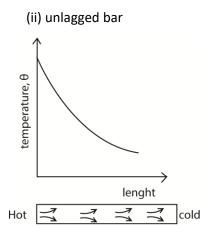
The rate of heat flow decrease with length due to heat losses
