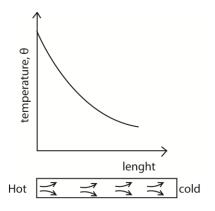
The rate of heat flow decrease with length due to heat losses
