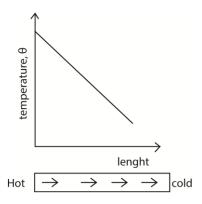
The rate of heat flow along the bar is constant since heat loss is negligible.
