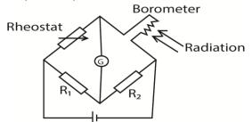
The bolometer strip is connected to Wheatstone bridge circuit above. The rheostat is adjusted until the galvanometer shows no deflection. When the radiations fall on the strip, they are absorbed and its temperature rises leading to an increase in resistance. The galvanometer deflects showing the presence of radiations.
