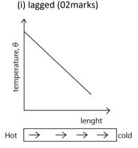
The rate of heat flow along the bar is constant since heat loss is negligible.
