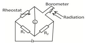
The bolometer strip is connected to Wheatstone bridge circuit above. The rheostat is adjusted until the galvanometer shows no deflection. When the radiations fall on the strip, they are absorbed and its temperature rises leading to an increase in resistance. The galvanometer deflects showing the presence of radiations.
