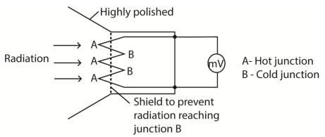
Radiation falling on junction A is absorbed and temperature rises above that of junction B. An e.m.f is generated and is measured by millivolt meter which deflects as a result.
