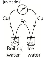
The e.m.f,  $E_{Tr}$  is obtained when a hot junction is placed in water at triple point. E.m.f,  $E_T$  is obtained at unknown temperature T.
