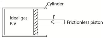
A fixed mass of an ideal gas is confined in a cylinder by frictionless piston of cross section area A. the piston is in equilibrium under the action of force, F as shown in the figure above. Show that the work done, W, by the gas when it expands from  $V_1$  to  $V_2$  is given by
