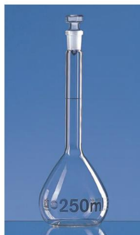
Volumetric flask measure precise volumes
