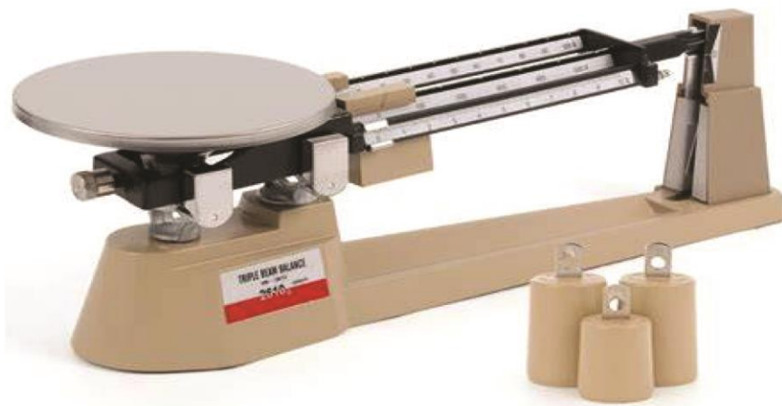
Beam balance for weighing mass
