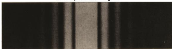
Diffraction band formed by a single small rectangular aperture
